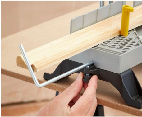
1. Attach the clamp to the workbench.
