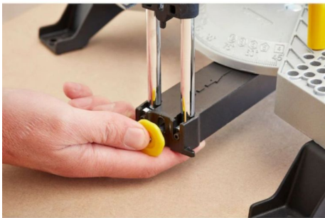
2. Adjust the clamp to the desired position.
